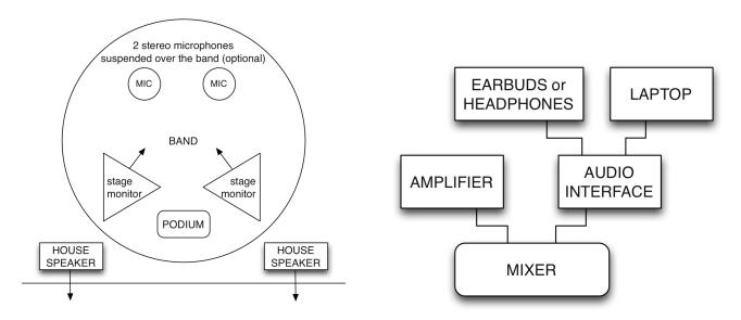
Monitors, speakers, laptop, audio interface, and microphones, if desired (not needed), are connected by cables to the mixer, which is usually centrally placed in the back of the auditorium, or otherwise, on the side of the stage. It's helpful to also have one or two stage monitors at the rear of the stage, so that the percussionists can clearly hear the pulse of the track.
