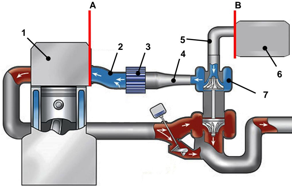
**A** Connection for compressed air adapter cap or sealing cap
