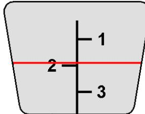
The scale behind the viewing window (4) is used for setting the integer values (1 Nm, 2 Nm, 3 Nm, etc.).
