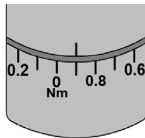
Digits after decimal point can be set in increments of 0.1 Nm using the scale (5) at the setting wheel.
