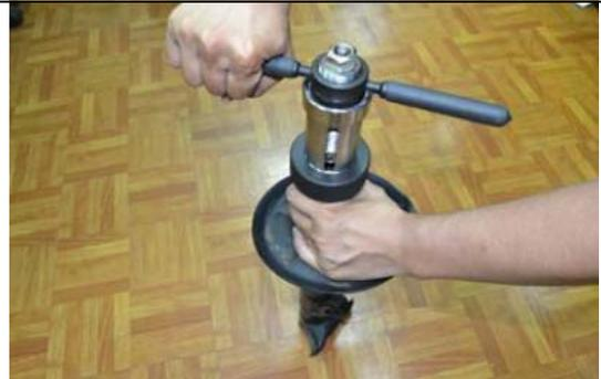
Tighten the clamp in the "tensioned" position.
