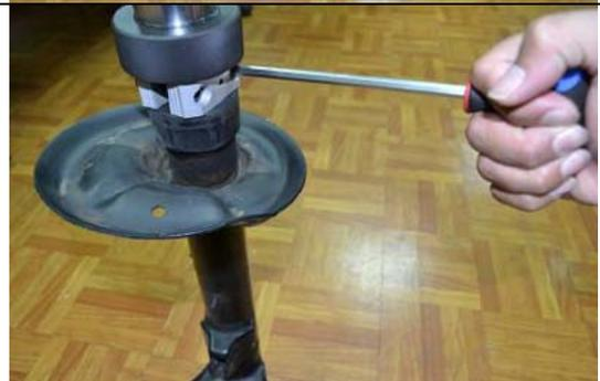
Remove the puller and mount the spring and spring plate.
