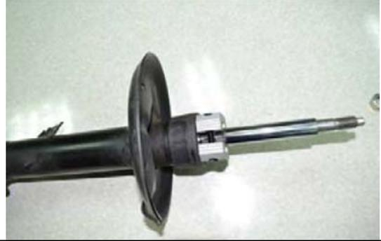
Put the puller device on the strut and lock the nut.
