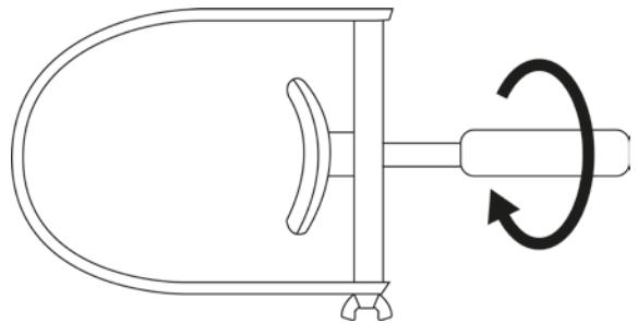
The internal diameter of the wrench can further be reduced by using the adjustment holes at each site of the device.
