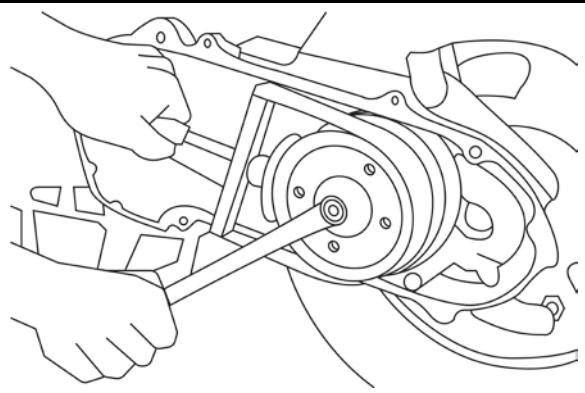
Use an appropriate wrench and socket to loosen the pulse wheel nut while holding it in place with the wrench.
