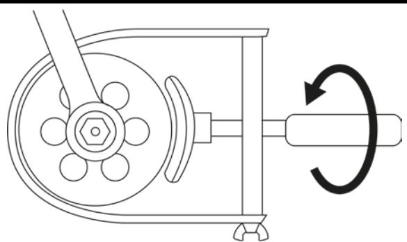
Fix the wrench on the clutch basket by turning the T-bar handle clockwise.
