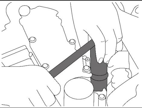
Remove the electromagnet of the injector.
