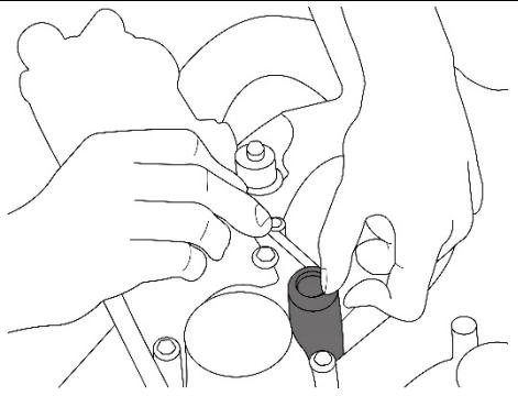
Pressing down the cloverleaf-shaped washer and remove retaining clip.
