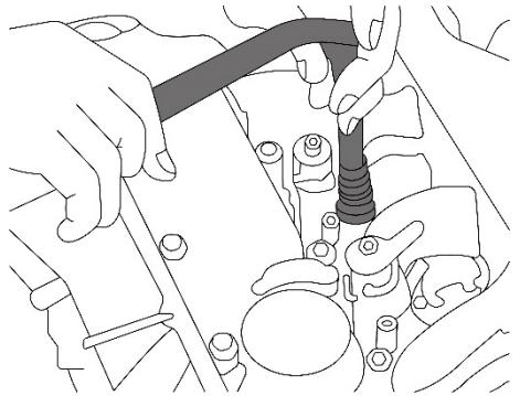
Remove the securing screw of the injector.
