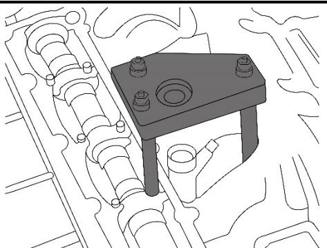
Screw the pulling spindle through the bridge into the injector.
