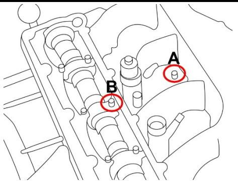
Place the support bolts in the holes in the intake manifold and in the screw of the bearing cover , as shown in the illustration.
