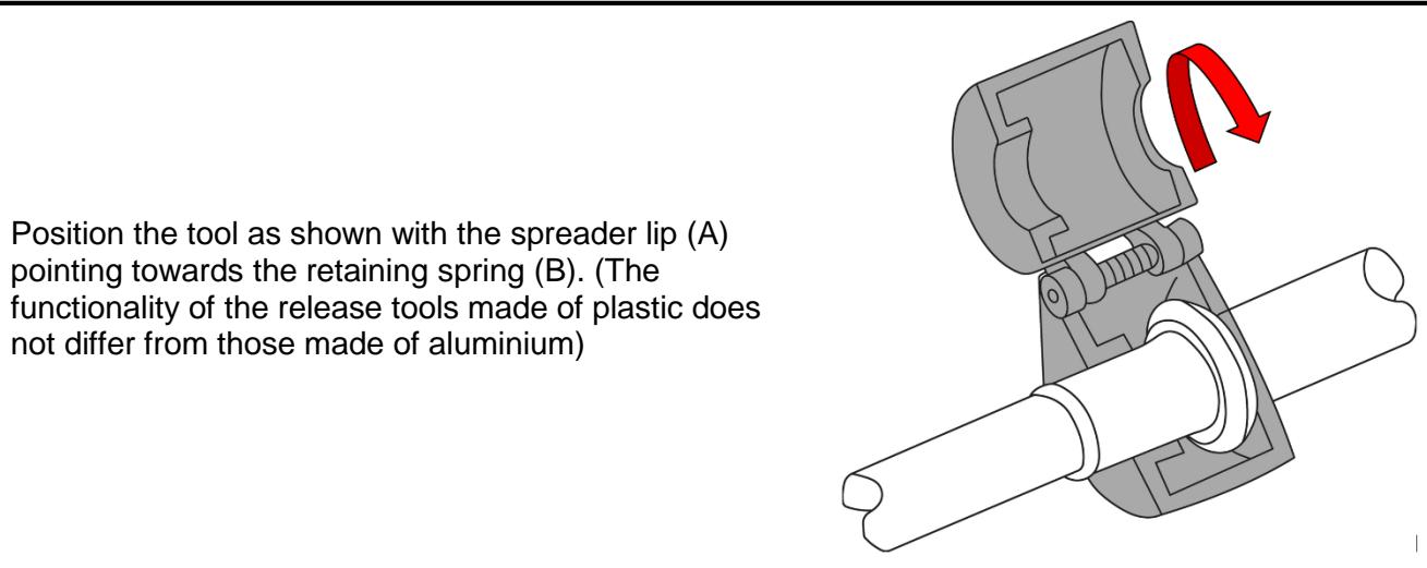
Position the tool as shown with the spreader lip (A) pointing towards the retaining spring (B). (The functionality of the release tools made of plastic does not differ from those made of aluminium)
