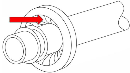
The retaining spring (B) serves as a locking device and holds both pipe ends together. This spring needs to be braced for a disassembly.
