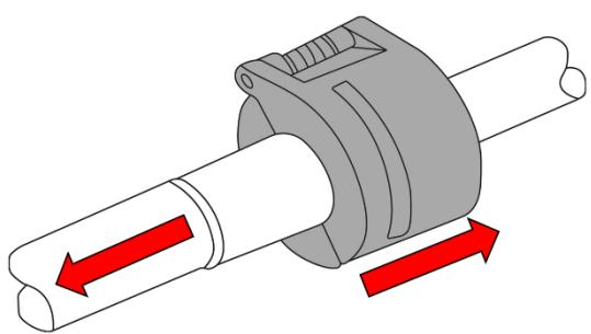
Push the removing tool against the pipe connector's retaining spring and pull the pipes apart.
