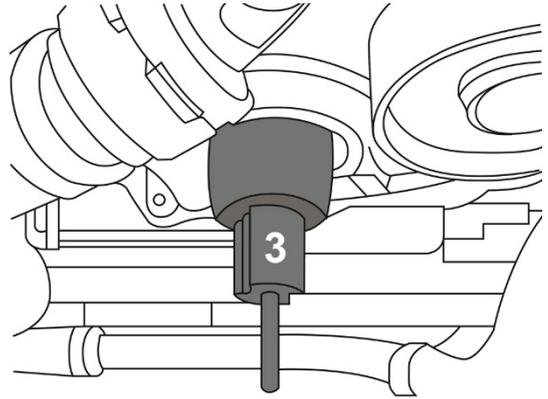
Push the new crankshaft radial sealing ring (A) carefully and straight onto the centering tool (3) with a rotating movement until the sealing ring is flush with the crankcase.
