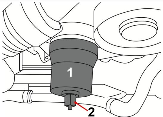
Press the crankshaft radial sealing ring into the crankcase via the thrust sleeve (1) by turning the nut (2).
