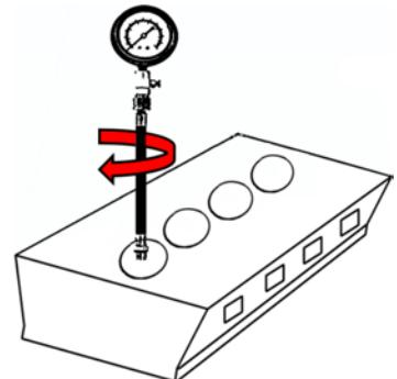
5. Now start the engine for about 4 seconds until the pressure on the tester no longer rises.
